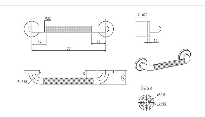
Other lengths available: 305mm, 406mm, 610mm, 914mm, 1066mm, 1219mm Mounting Formats: Threaded Flange ("TF") or Snap Flange ("SF")
